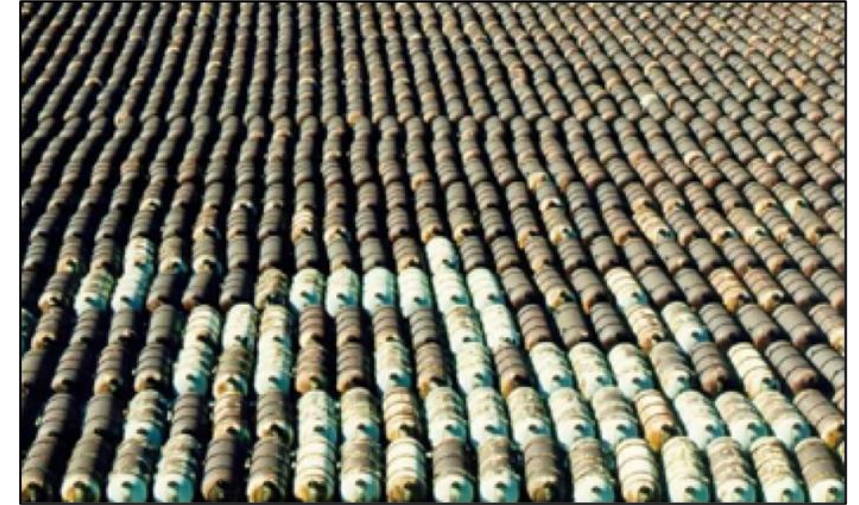
Depleted UF6 Tails stored in Ohio, USA
