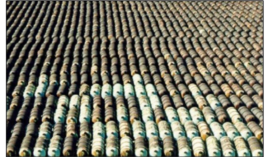
Depleted UF6 Tails stored in Ohio, USA
